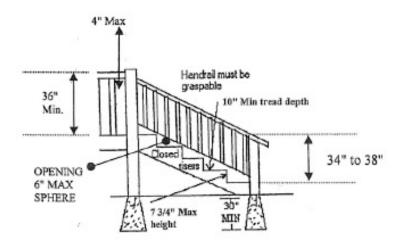
All footings/piers for posts must be at least 30" below grade and a minimum of 12" wide (diameter) Belled 18" wide (diameter) at the bottom for frost protection.
